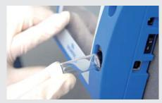
**1.** Start test by determining the background value of cuvette
