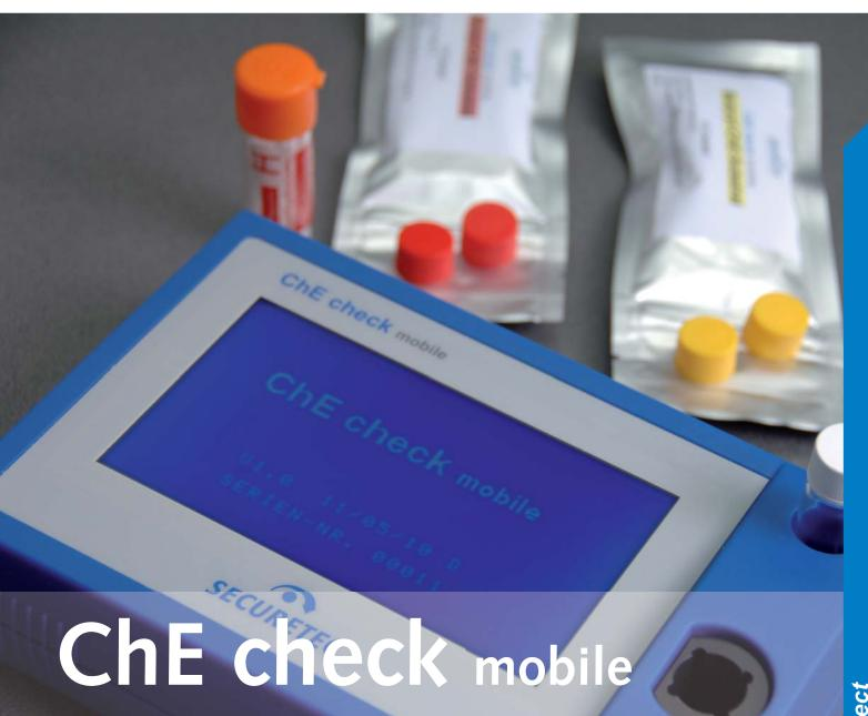
Portable cholinesterase testing system
