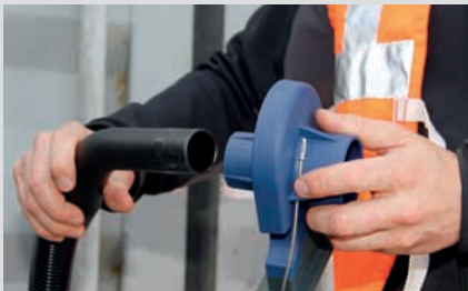
3. Assemble the vacuum tube to the cartridge case.
