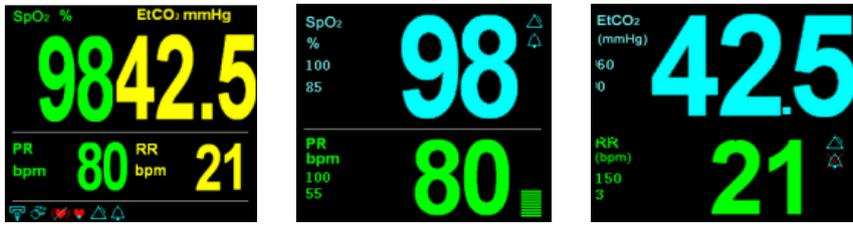
(a) SpO<sub>2</sub> and CO<sub>2</sub> Module (b) SpO<sub>2</sub> Only (c) CO<sub>2</sub> Only
